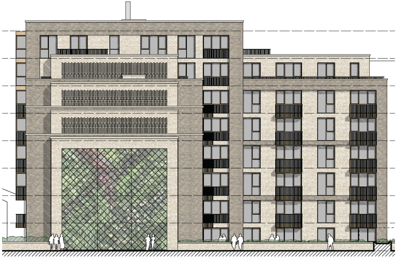
Fig. 9. Amended rear elevation to include raised brick bond pattern on rear elevation.
